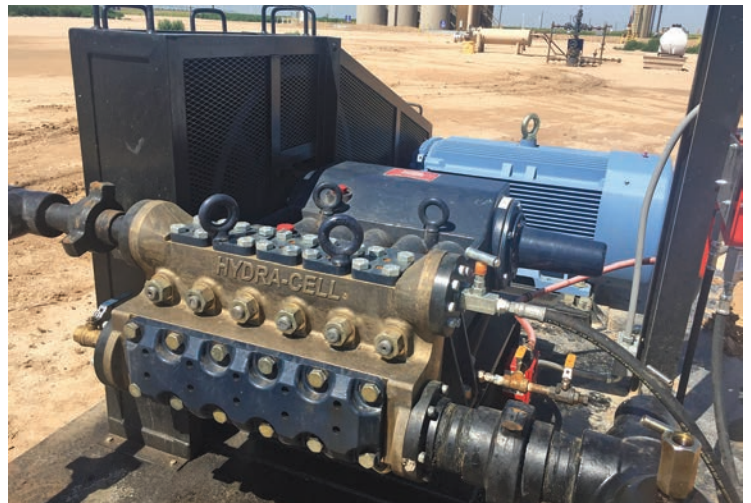
T and Q Series pumps feature the Hydra-Cell seal-less design, eliminating clean-up costs from leaking seals or packing and protecting operators from dangerous fluids such as those containing hydrogen sulfide (Q155 shown).
