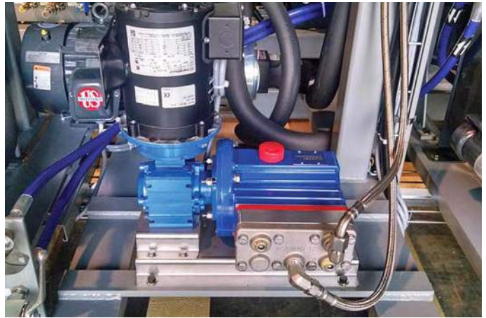
A P200 replaced an external gear pump to deliver a catalyst for polyurethane foam production and doubled volumetric efficiency.
