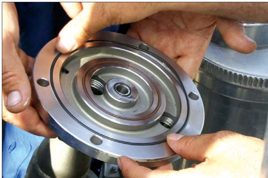
Simple build, low maintenance. This Hydra-Cell pump manifold inspected by Romgaz engineers after 1800 hours continuous operation showed no signs of wear.
