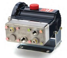
A Hydra-Cell model D03 used to pump a Nitroglycerin slurry is equipped with hydraulic variable speed drive to provide 0.7 to 1.1 gpm constant flow over a pressure range of 75 to 175 psi. The duty cycle is 2 or 3 hours per day with an operating temperature of 70°F.
