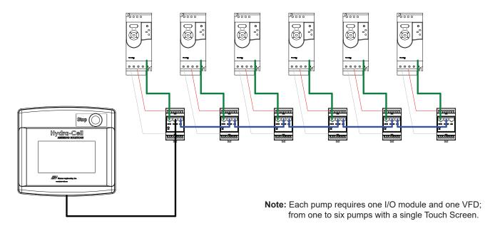
Single Touch Screen Multiple Pump Networking Wiring Diagram
