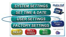
Enter Model #, Motor RPM, and System Pressure for your pump.
