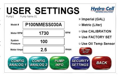
Note: The Model #, Motor RPM, and System Pressure entries are used to provide maximum metering accuracy.
