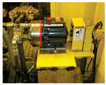
Hydra-Cell providing dust control on a rotary drilling machine.
