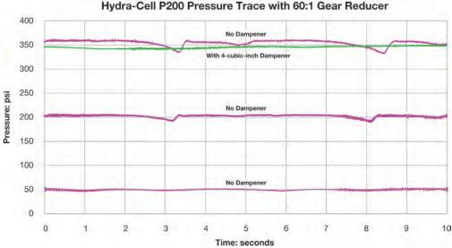
Hydra-Cell P200 Pressure Trace with 60:1 Gear Reducer
