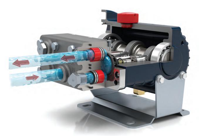
Abrasive particles and slurries can cause wear to dynamic seals and damage other types of pumps. Hydra-Cell's seal-less design and horizontal check valve orientation will handle abrasives and particulates without clogging or damaging the pump.
