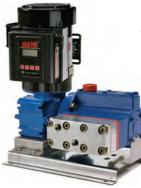
Hydra-Cell metering pump Weight: 83.5 lbs. (with motor) Rated: 2500 psi at 36 gph Motor: I-1/2 hp
